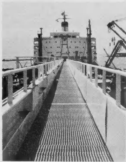
LOOKING AFT over the catwalk of the Esso Lincoln places a long expanse of steel between the viewer and ship's accommodations. This is the first Esso ship to have all quarters aft and nothing forward. MIRANDO PATRAS over di e catwalk di Esso Lincoln ta keda un distancia grandi di staaal entre e mirador y e acomodacionnan di e bapor. Esaki ta e promer bapor Esso cu tin tur camarote patras y nada padilanti.
